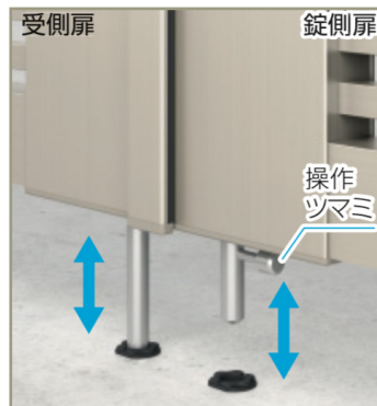
Lock-down stick on the main panel (moves first) is activated by turning and pulling down the stick
